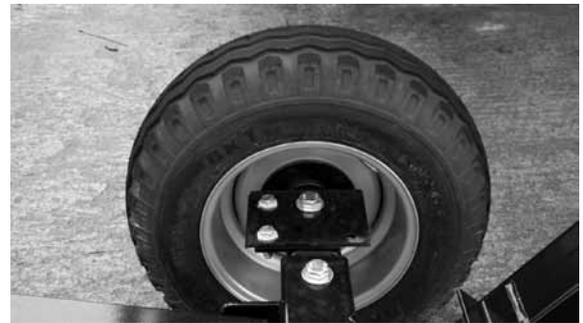
Radial wheel standard for maximum stockpiling
